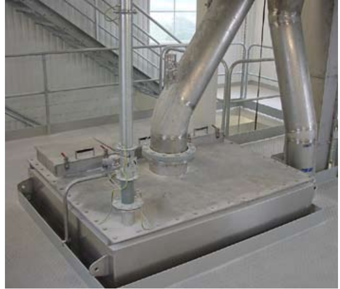
TOP VIEW OF INLET HOPPER
