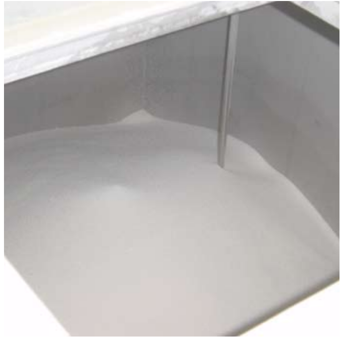
R.A.R – Sugar Inside Cooler and Level Probe
