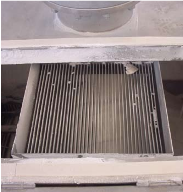
Danisco – Coarse Screen Inside Inlet Hopper
